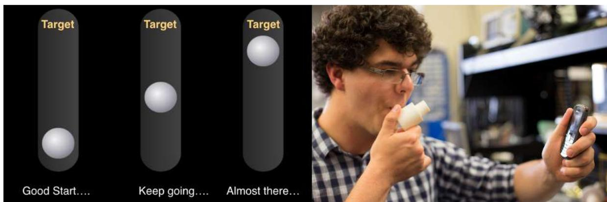
Figure 6.2: **(left)** As a person pushes more air out of their lungs, the ball in the SpiroSmart visualization rises to the top and encourages to the user to continue the maneuver. **(right)** The SpiroSmart vortex whistle can be used to control the diameter of the user's mouth, acting as a flow-to-pitch transducer.
