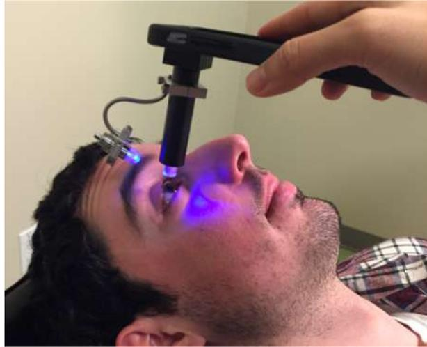
Figure 3.1: The proposed system emulates fixed-force applanation tonometry using the hardware adapter pictured above. The clear acrylic cylinder is allowed to move freely within the black casing so that its mass provides a constant force on the patient's eye.
