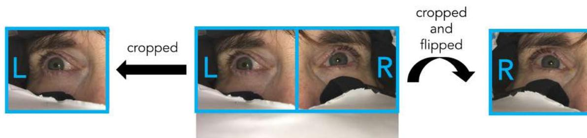
Figure 5.6: Each frame was cropped to create two input images for the CNNs: one for the left eye and one for the right eye. The image of the right eye and its label were flipped to make the two images comparable.
